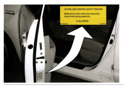
Figure 1 Vehicle load label
