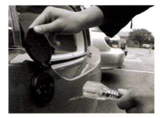
Figure 5 L5 PCM charge port location
