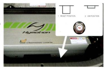
Figure 7 L5 PCM circuit breaker
